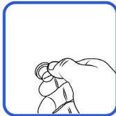
6. Screw on the reset button cover.
