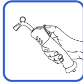
2. Press the steam button on the steam gun until the pressure drops to zero.
